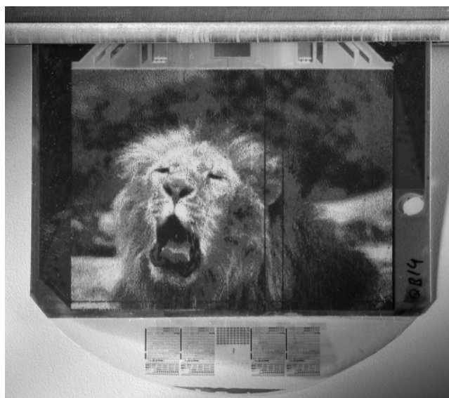
Figure 7. Finished electrophoretic quarter-VGA display with a flexible AM-OTFT backplane patterned by photolithographic processing. Photograph courtesy of Polymer Vision ( www.polymervision.com ).
